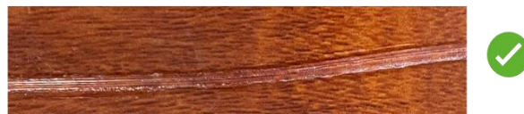
Cabling too fast, adhesive not fully melted
