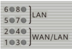
Figure 4-2 Silkscreen indicator area 2
