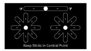
2. Release the rocker and the gimbal pitch angle thumbwheel to return them to the center position naturally. The three center dots on the calibration screen of the remote controller will be highlighted in turn.
