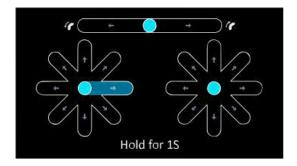
4. Push and hold the **rocker** in eight directions one by one until you hear a beep. Then turn the **gimbal pitch angle knob** clockwise until you hear a beep, and turn it counterclockwise until you hear a beep.
