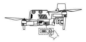
**4.** Press and hold the power button ( ) and return button ( ) for 2s at the same time until "Autel"shows on the flight information panel. After pairing is successful, the pairing indicator on the aircraft will turn off.
