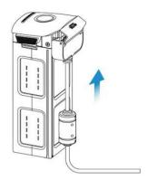
Remote controller: Open the protective cover of USB port, and insert the charge wire provided.
