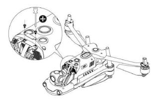
3. Insert a screw into a hole of the gimbal decorating part, and then screw it with a T6 screwdriver until the screw is fixed but not being tightened. Repeat this step for other screws. Fully tighten the two screws with the screwdriver.
