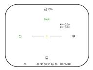
Distance: Adjust the distance of 10m by rotating the wheel.
