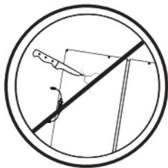
This Solar Panel contains **glass** inside. Behaviors above that damage the solar panel, will cause the glass inside the solar panel to crack and efficiency drop, or even unusable.
