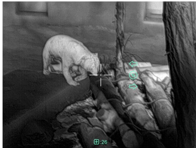
Fig. 6-3 Blind pixel correction interface
