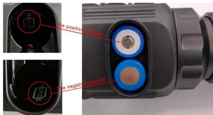
Fig. 8-1 Schematic diagram of battery installation
