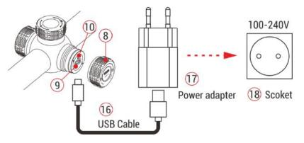
**Note:** It only supports charging the built-in battery pack, not the replaceable 18500 battery.
