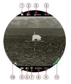
The status bar is located at the top of the image interface and displays the information related to the current operating status of the device.
