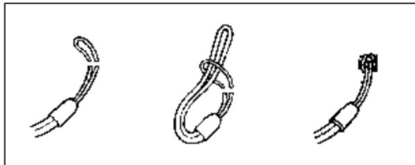
Feed the small loop on the carry strap through the eyelet **4** on the housing of the Leica Rangemaster. Then thread the end of the strap through the small loop created and pull tight, so that the resulting loop is secured on the eyelet on the housing.
