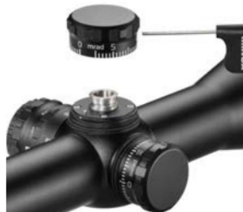
\* If after installing the FRA it should become necessary to re-zero your riflescope, it may be necessary to temporarily loosen and retighten the FRA turrets at a different position to bypass the integrated end stops. After re-zeroing, the FRA turrets can be set and tightened at the „zero“ index marks again.
