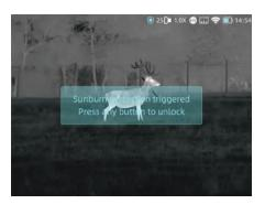
Once it detects harmful rays to the detector, the system will enable protection automatically.
