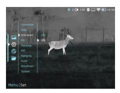
Detector anti-burn function, it could be set by on/off.
