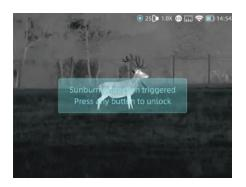
Once it detects harmful rays to the detector, the system will enable protection automatically.
