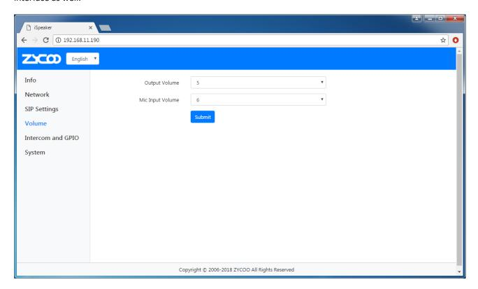
There are 10 levels of the audio output volume and microphone input volume.
