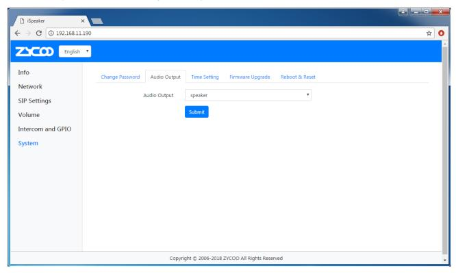
In Speaker mode, you may connect loud speakers/passive speakers to the "Speaker" interfaces, the output power is up to 2x10W(dual-channel),  $8\Omega$  impedance.
