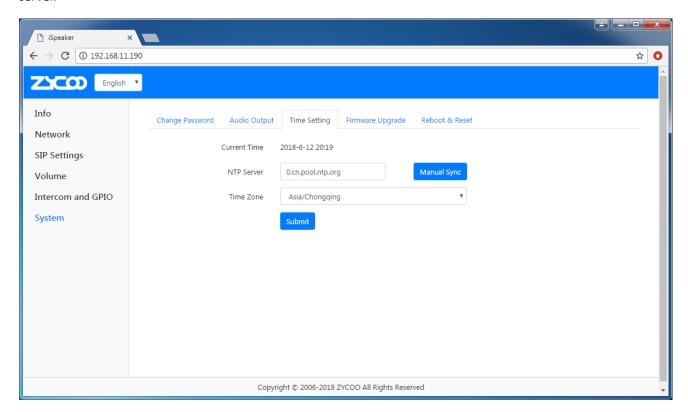
On the Time Settings screen, you may check the current time, if it's not correct you may click on the "Manual Sync" button to synchronize time from the NTP server (please ensure X30 has network connectivity), if the default time zone is in the different zone as yours please change the time zone and then synchronize the device time from NTP server.
