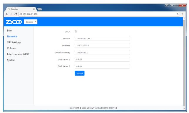
Changing network profiles requires restarting the device, please click on "Reboot" button to restart the device and after 40 second you may access it via the new IP you have configured.
