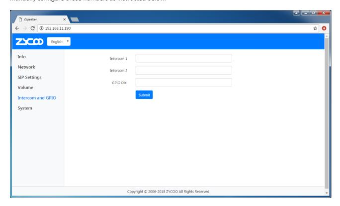
As shown in the screenshot above, in "Intercom1" and "Intercom2" field, you can configure the intercom number directly, when one of those keys is pressed, intercom call will be made to the configured number.
