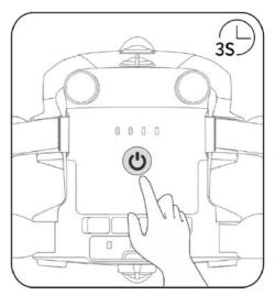
Fig 5-2 Turn On or Off the Smart Battery
