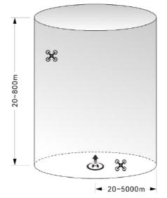
Fig 2-5 Diagram of altitude and distance limits
