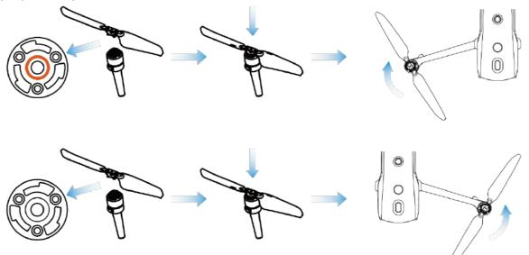
Fig 3-5 Install the Propellers
