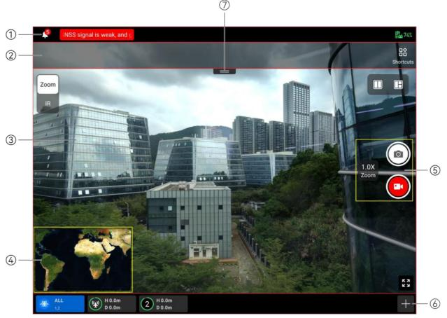
Fig 6-1 Main Interface of the flight application (Fusion 4T/4T XE Gimbal and in A-Mesh Link mode)
