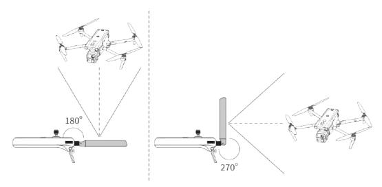
Fig 4-10 Extend the antenna
