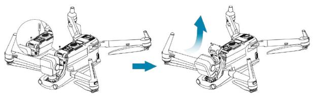
Fig 3-13 Removing the Gimbal
