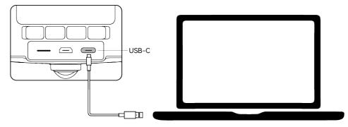
Fig 3-16 Connect to PC/MAC via Aircraft USB-C interface
