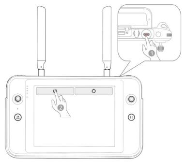
Fig 4-7 Turning the Remote Controller Off
