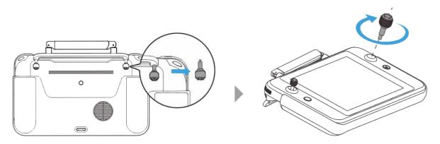
Fig 4-5 Installing sticks
