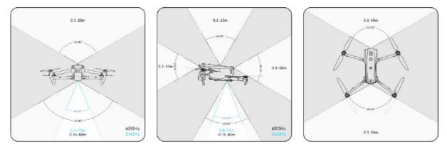
Fig 2-4 Observation Range of Millimeter-Wave Radars
