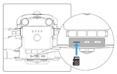
Fig 3-15 Installing the microSD Card
