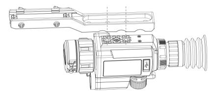
Figure 2-5 Align Installation Holes
