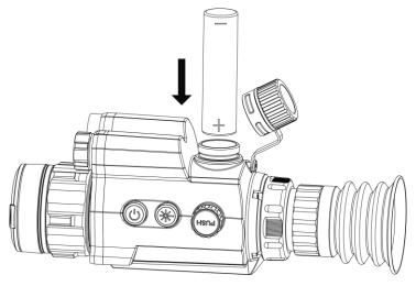
Figure 2-3 Install Battery
