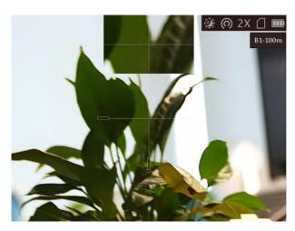
Figure 4-2 PIP Effect in Reticle Mode
