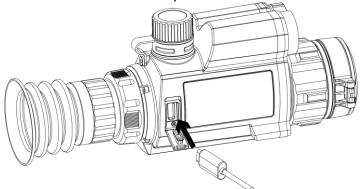
Figure 2-1 Cable Connection
