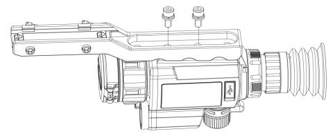
Figure 2-6 Install Screws
