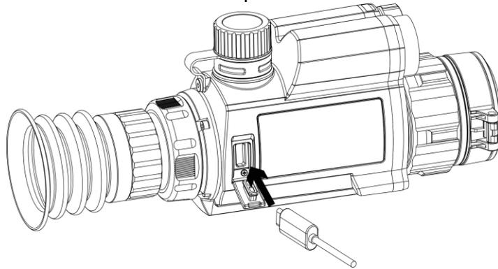
Figure 2-1 Cable Connection
