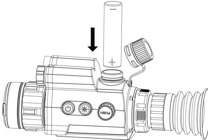
**Figure 2-3 Install Battery**
