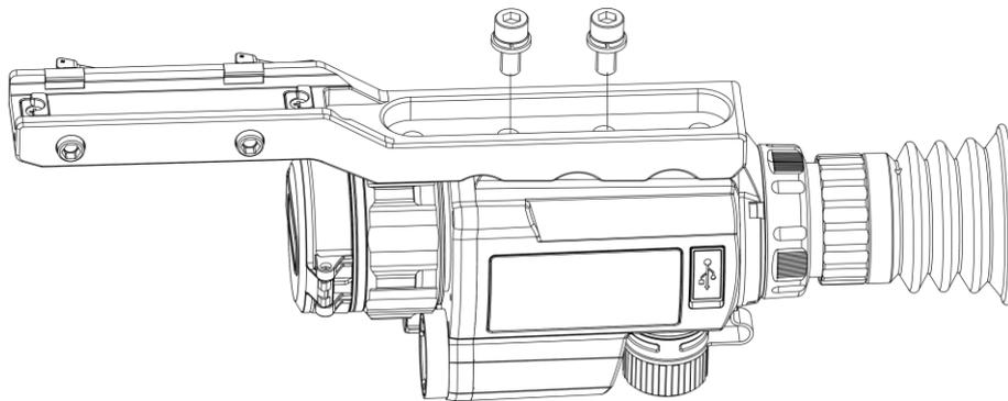
**Figure 2-6 Install Screws**
