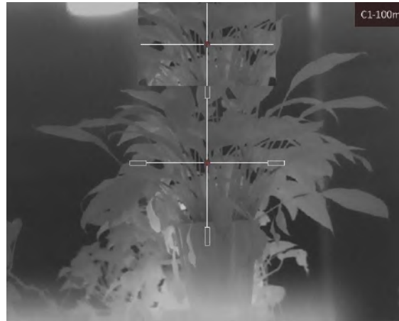
Figure 4-2 PIP Effect in Reticle Mode
