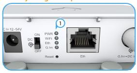
Verify basic Bridge AP operation by checking the system LEDs.
