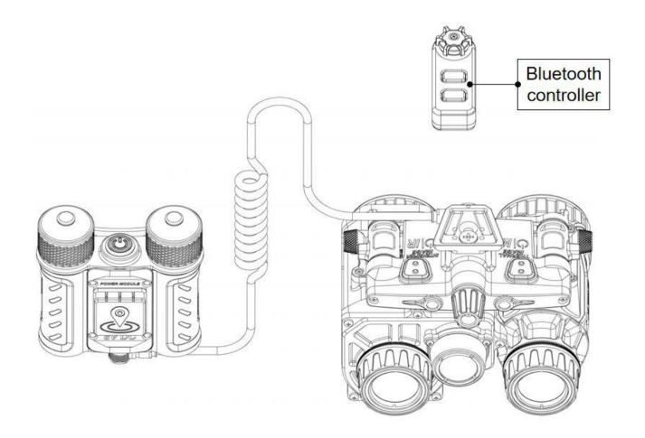
The external Bluetooth controller can control and adjust the host of the night vision instrument. Please set and adjust the remote controller through the "MENU-SENSOR-BT". The Bluetooth remote controller has a sleep function. When the controller is not operated, it will automatically enter low-power sleep. Please click the middle button to wake up.
