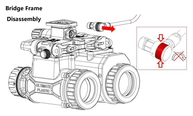
Please press and hold the cable head to remove the connecting cable(The red position is the lock ring). Do not use the knob connector, otherwise the device will be damaged
