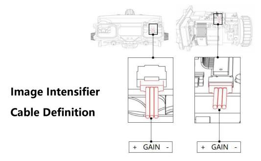
Support contact type, 2-wire and 3-wire image tubes
