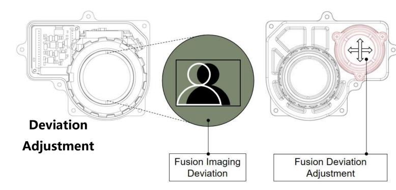
If there is deviation between Thermal Image and Image Intensifier after installation, Please loosen the flange screw (M1.6-3pcs) and move the infrared lens flange to adjust the deviation, or fine tune the calibration through the MENU -SET-Deviation
