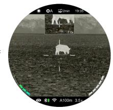
hold the Image Mode button (6) to turn on the PIP function.
