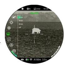
When using the scope, you may see pixel defects, such as visible light spots or dark spots with stable brightness. To address this problem, use the Pixel Defect Correction function to remove the pixel defects.
