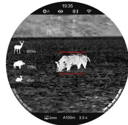
reduce the width of the measurement lines, so that the target is completely between the measurement lines.
