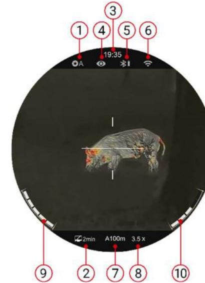
The status bar is located at the top of the image interface and displays the information related to the current operating status of the device.
