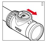
A 3 V lithium coin cell (type CR 2032) is required for power supply.
