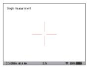
When under real time image mode, Long press **Down** Button to enter/exit scan mode. Aim  $\frac{1}{100}$  to the target, the corresponding distance of target will appearson display.
