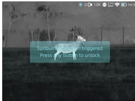
Once it detects harmful rays to the detector, the system will enable protection automatically.
