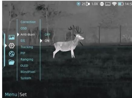
Detector anti-burn function, it could be set by on/off.
