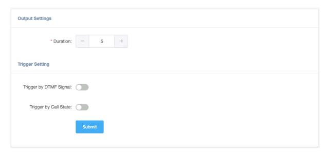
The switch signal output duration can be configured from 1 to 600 seconds.
