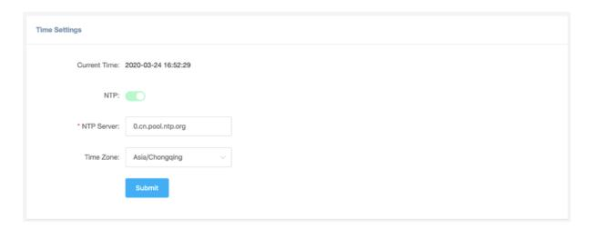
Here you can change a NTP server by modify the NTP server address and you can select the time zone of your location, so the network speaker will synchronize time of your time zone from the NTP server you have configured.
