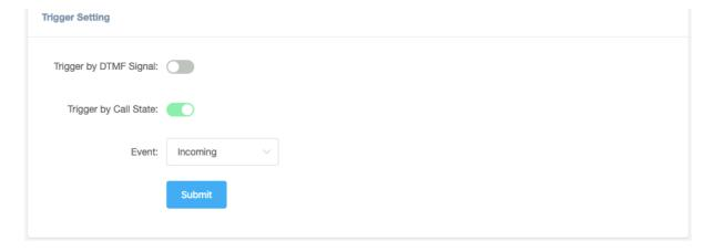
If "Incoming", the dry contact relay output will be triggered when the network speaker gets an incoming SIP call (paging).
