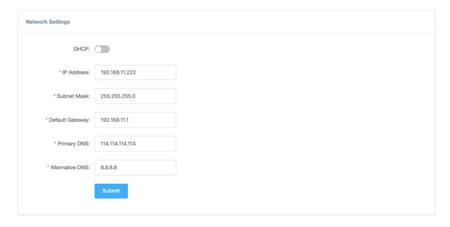
Turn the DHCP switch button off to show the network parameter settings.
