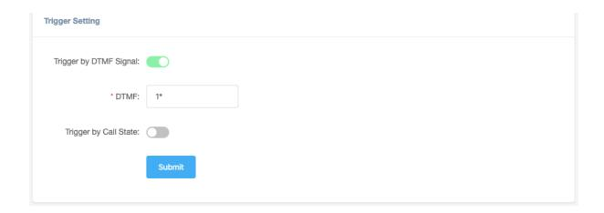
In this example, DTMF key press is \*1, so during a SIP call (paging), the caller press \*1 from the phone key pad, it will trigger the dry contact relay output on the network speaker.
