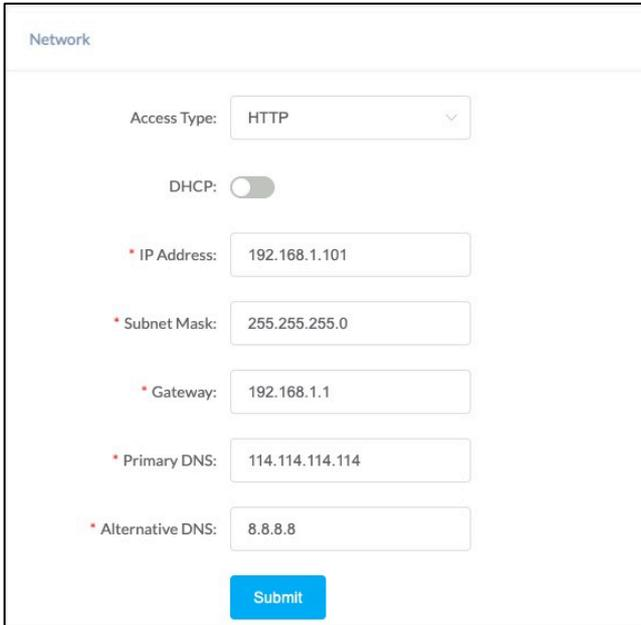
The screenshot shows the 'Network' settings page. At the top, 'Access Type' is set to 'HTTP'. Below it, the 'DHCP' toggle switch is turned off. The static IP configuration fields are as follows: IP Address: 192.168.1.101, Subnet Mask: 255.255.255.0, Gateway: 192.168.1.1, Primary DNS: 114.114.114.114, and Alternative DNS: 8.8.8.8. A blue 'Submit' button is located at the bottom of the form.
