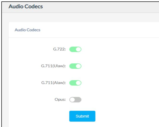
The screenshot shows the 'Audio Codecs' configuration page. It has a title bar 'Audio Codecs' and a sub-header 'Audio Codecs'. Below are four rows, each with a label and a toggle switch: 'G.722:' with a green toggle, 'G.711(Ulaw):' with a green toggle, 'G.711(Alaw):' with a green toggle, and 'Opus:' with a grey toggle. A blue 'Submit' button is centered at the bottom.
