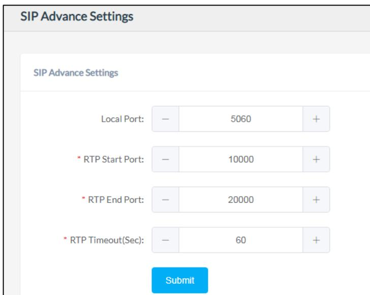
The screenshot shows the 'SIP Advance Settings' configuration page. It has a title bar 'SIP Advance Settings' and a sub-header 'SIP Advance Settings'. Below are four rows, each with a label and a numeric input field with minus and plus buttons: 'Local Port:' with value 5060, '\* RTP Start Port:' with value 10000, '\* RTP End Port:' with value 20000, and '\* RTP Timeout(Sec):' with value 60. A blue 'Submit' button is centered at the bottom.
