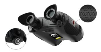
They are also ergonomic for use outdoors — the placement of the focal rings close to the thumb and the anti-slip handle ensure smooth operating and effectively alleviates the fatique arising over extended periods of use.
